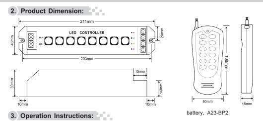
8 function buttons on the receiver, which is corresponding to the first 8 button on the remote: namely ON/OFF, PAUSE, MODE+,MODE-, SPEED+,SPEED-, BRT+,BRT-.
