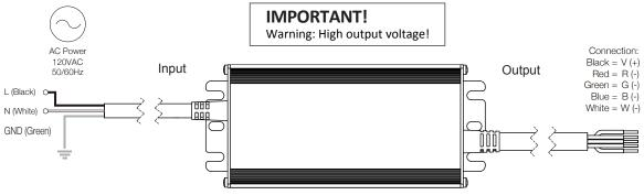
For single white LED strip, max. current: 2.17A, max. load power: 260W For RGB LED strip, total max. current: 5.17A, total max. load power: 620W See fixture specifications for maximum series run limits.
