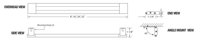
Note: Ambient operating temp range -4F to 104 F. Do not install in an environment that is outside of the product's listed ambient temp.
