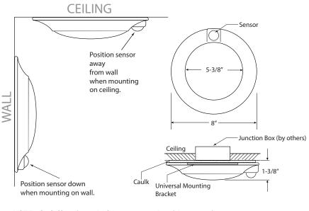
NOTE: On/off activated after 30 seconds without motion. To maintain wet listing, fixture must be sealed with caulk.
