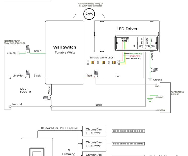
Note: All drivers will work in sync. (1) Wall Controller can pair with (6) drivers max.
