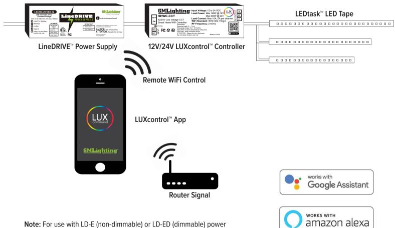
**Note:** For use with LD-E (non-dimmable) or LD-ED (dimmable) power supply only. Not compatible with LD-MD (magnetic) power supply.
